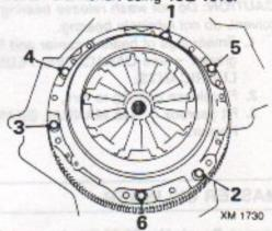
Tighten 6 bolts progressively in order shown to 22 Nm.
