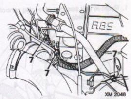
Release slave cylinder feed pipe from 3 clips; move pipe aside.
