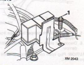
Remove bolt securing glow plug control unit; move unit aside.
