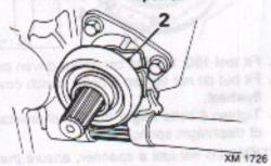
2. Remove release bearing from fork.
