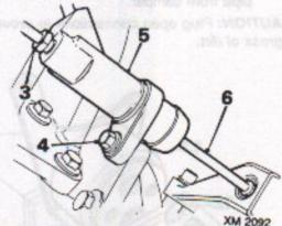
Disconnect feed pipe from slave cylinder.
