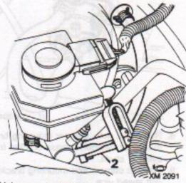
Using a suitable hose clamp, compress master cylinder feed hose.
